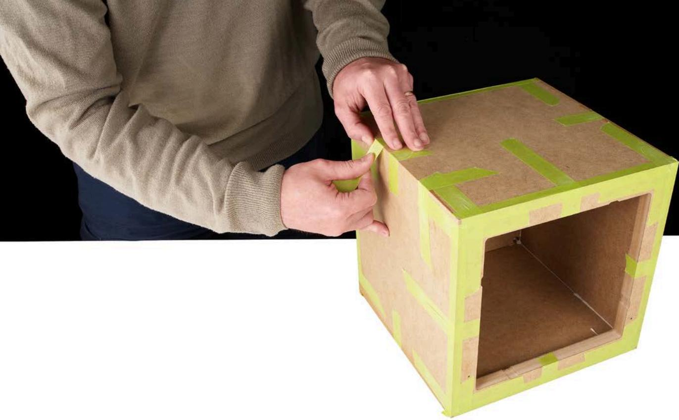
Wipe excess glue and secure with masking tape. Use firm pressure when applying the tape. The tape holds the panels together as the glue sets and should cover all joints.
