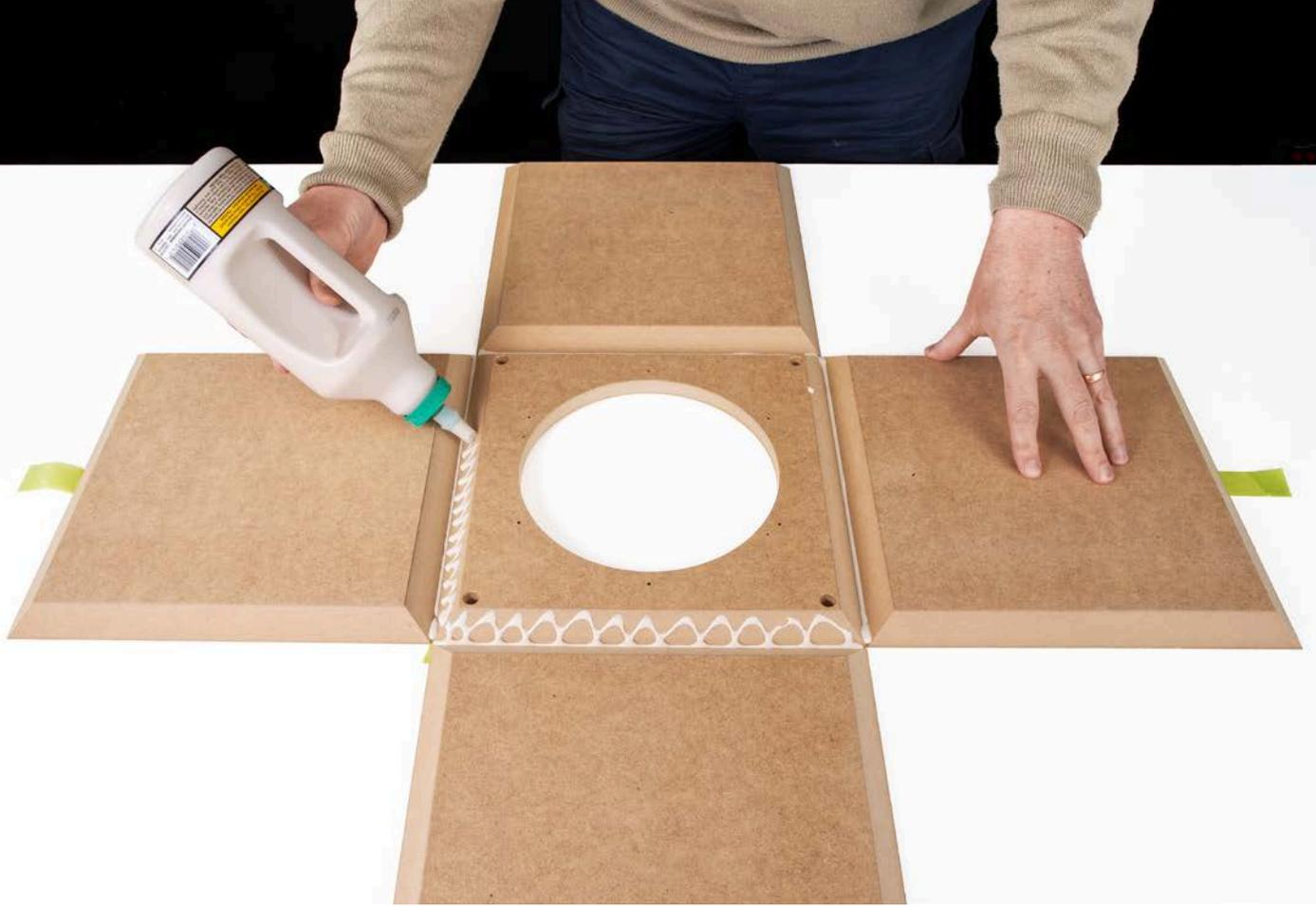
Apply glue in a zig zag pattern to cover the mitre. Confirm that the glue adequately covers the entire surface of the joints by folding up each pair of panels.
