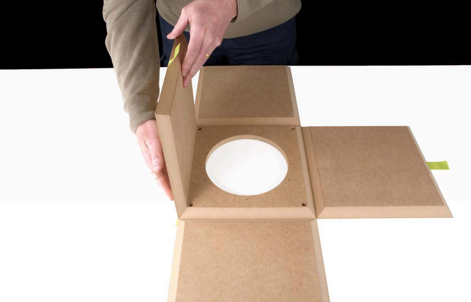
Now rotate up each of the four panels and firmly press the masking tape onto the join to ensure good adhesion, as shown above.
