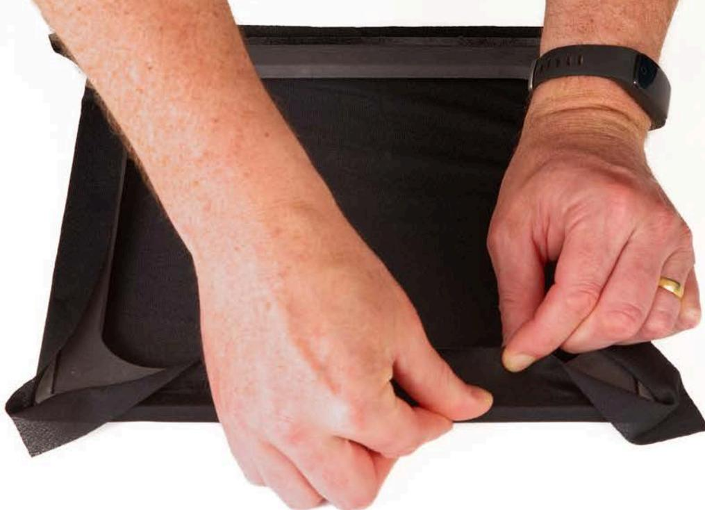
Now press the grille cloth to the frame on the third side, avoiding contact around the corner. Then finally, press the cloth to the final side of the frame. In this step, all wrinkles from the tension should be gone.
