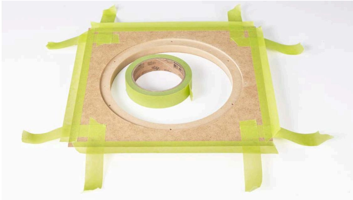
Flip over the panel to expose the mitres. Carefully position the four adjacent panels and press firmly each panel along the join to adhere the tape, as shown below.
